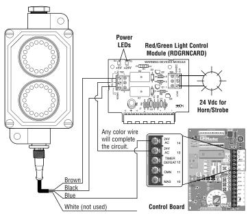
**NOTE:** In most cases the Traffic Light can be powered by the operator's transformer. If multiple accessories are powered by the operator, such as 2 sets of Traffic Lights and photoelectric sensors, a transformer upgrade may be required. (See Transformer Upgrades below.) A 460 V operator will not require a transformer upgrade.
